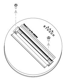
At the front of the monopoint adapter, remove the two screws.
