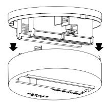
Remove the bottom housing from the adapter.
